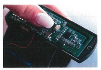
2. Press and hold the button on the receiving card.
