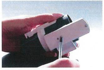
1. Open the door of the Flisy 2 receiver module by unscrewing the screws with a star screwdriver.
